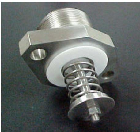
Heavy duty, variable orifice hollow cone spray nozzles are constructed of Stainless Steel with a Teflon spreader, to eliminate all metal to metal contact and wear.
