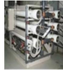
Continuous high purity effluent for process and boiler feed. Altair reverse osmosis systems utilize low pressure energy efficient thin film membranes for longevity and low cost operation. 99% rejection. Single and double pass systems with PLC controls, welded steel frames. Altair reverse osmosis systems offer as standard features many of the components and features that are optional on other manufacturers systems.
